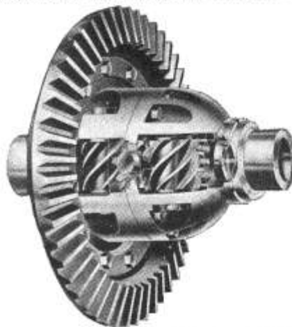
An imaginary illustration of the automatic differential-locking gear on the Muehl system.
